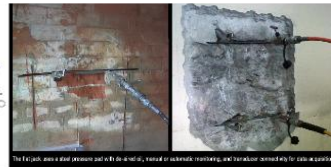
The flat jack, also a steel pressure pad with de-aired oil, manual or automatic monitoring, and transducer connectivity for data acquisition.
